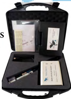
Easy onsite measurement on your tablet or laptop with the handy calibration field case supplied in the pack
