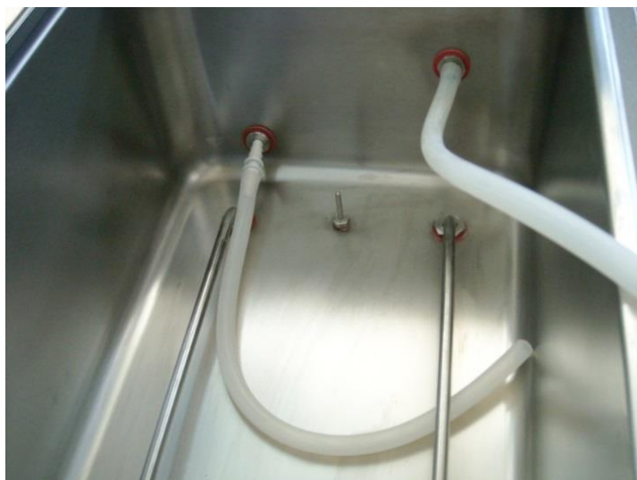
Picture 4 – Emptying kit for water bath with pump
